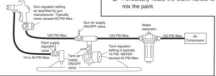
Figure 5. Paint tank connect to air compressor and spray gun.
